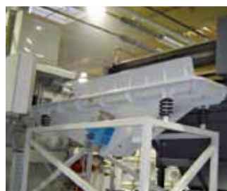
Transfer feeder with motor vibrators for continuous product transport between processes e.g. oil bath and washing system.
