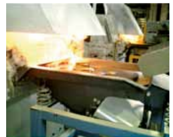
Transfer feeders made of heat-resistant steel for product feeding directly into furnaces with internal furnace belts.
