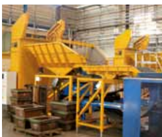
Complete furnace feeding system consisting of lift tipper, storage feeder including weighing system and vibratory transfer feeder for optimum automatic product feeding.
