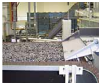
Automatic, consistent and optimum product loading on the furnace belt.
