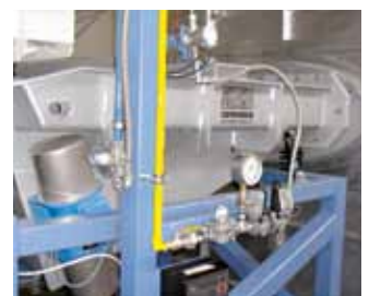
Transfer feeders with motor vibrators made of heat-resistant steel in an enclosed design with sealed flange connection.
