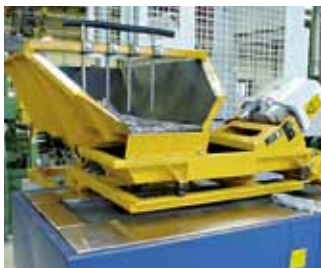
Special 'space saving' solutions including overhead electromagnetic driven units, allowing the transfer feeder to be installed directly above the furnace inlet.
