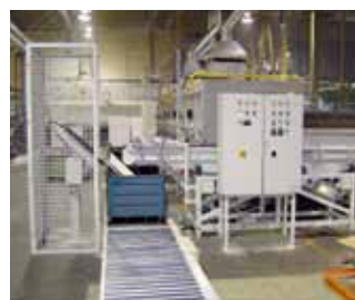
Gentle and automatic charging of containers after the tempering furnace, available with weighing function.
