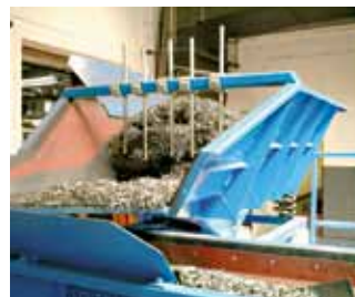
The combination of a storage feeder and vibratory transfer feeder allows for disentangling and automatic feeding of strongly interlocking products.
