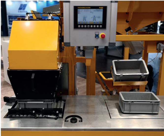
The standard system consists of a vibrating storage feeder, a vibrating conveyor, a chute system with accumulation possibility, a table with integrated load cells and a sample/check weighing platform.
