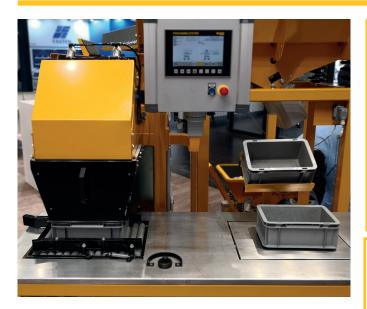
The standard system consists of a vibrating storage feeder, a vibrating conveyor, a chute system with accumulation possibility, a table with integrated load cells and a sample/check weighing platform.
