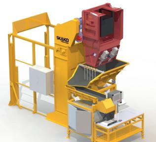
**OPTION:** Added Lift Tipper for safe & efficient charging of material into storage feeder.
