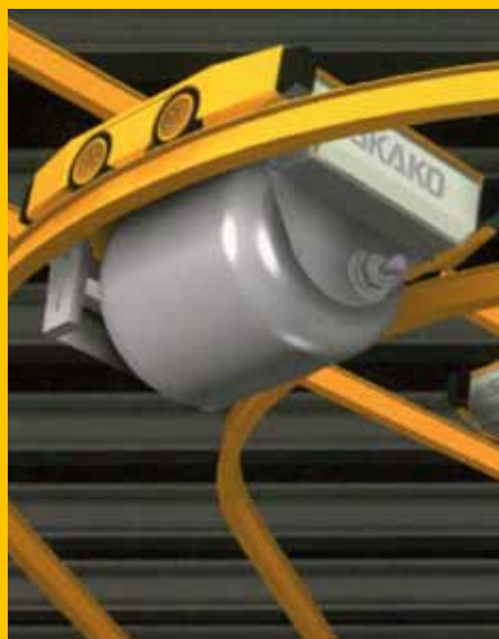
When turning, the CONFLEX uses a small radius of curvature.
