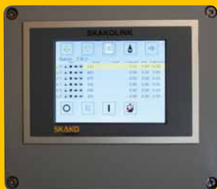
The control system controls up to 5 buckets, 30 work stations and 8 mixers.
