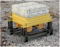
**THE MOVEABLE MINIGAB** Is a smaller version OF SKAKOGAB (1.000x1.000 mm), that easily can be transported from one site to another.
