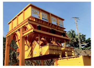
The stones can be discharged into the SKAKOGAB directly, or via a hopper with feeders that feeds into the SKAKOGAB. With the hopper solution, the filling of stones does not have to be timed, as the hopper can hold 4-5 filling cycles.
