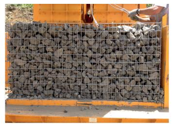
With the SKAKOGAB, the gabions are more compact, thus making them more stable. The weight of a 2m<sup>3</sup> SKAKOGAB gabion is appr. 3.600 kg, with a bulk density of 1,5. This is at least 10% more than a normal gabion.
