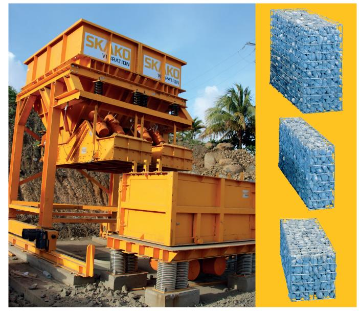
With the SKAKO patent pending system of filling gabions, the process of producing gabions is not only made faster, but also more efficient. The gabions become more compact, which is crucial when building retaining walls.
