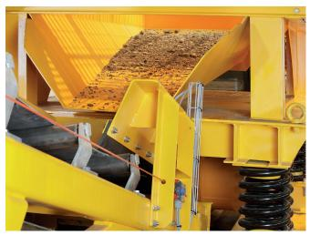
The metal bottom grate with discharge chute and belt conveyer facilitates the removal of fines, which minimizes the need for clearing the table in between crates.
