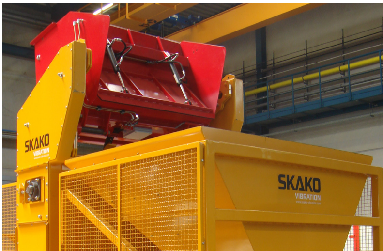
Heavy Duty designed "Jamming Free Guideway" for the "hoist chair" wheels included as standard.
