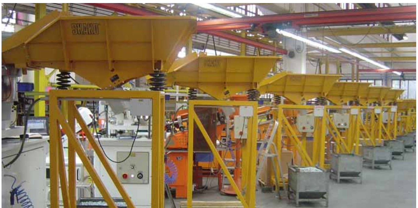
Multiple storage feeders loading thread rolling machines
