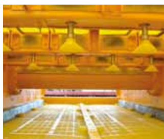
Spraying System To wash and rinse material
