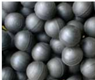
Deblinding Balls To prevent blinding of the screening deck
