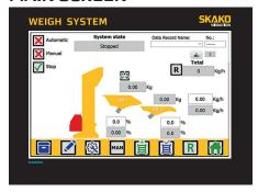
Visual overview of process. Easy access to adjust most common parameter. See total weight, number of weighings.
