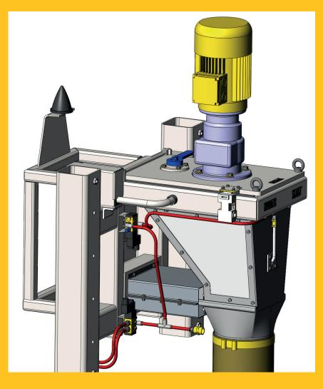
The compact unit consists of cutting head, outlet funnel with pneumatic sliding gate to prevent dust and moisture from penetrating the unit, and monitoring indicators of the rope in case of thread rupture or thread stop.
