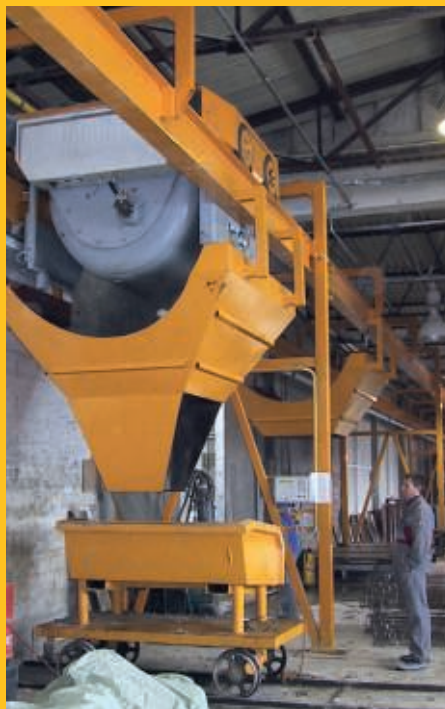
A SKAKO CONFLEX conveyor bucket arriving at work station.
